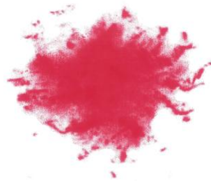
Figure 3. Scanned &amp; saved pressure measurement film (Low-type)
